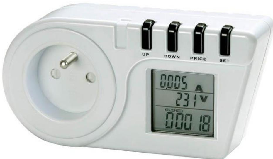
This plug is called a wattmeter or power meter. It is used to measure the power used by the different electric devices.
